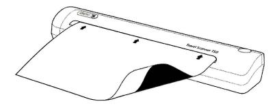
5. The scanner will pull the calibration page through the scanner. The page will move back and forth as the scanner calibrates for the difference between dark and light.
