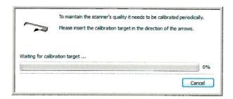
4. Place the calibration page in the scanner in the direction printed on the page. The black strip should be *face down*.
