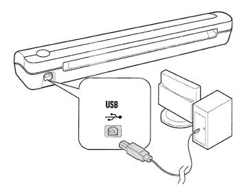
If the plug does not attach easily, make sure that you are plugging it in correctly. Do not force the plug into either connection.
